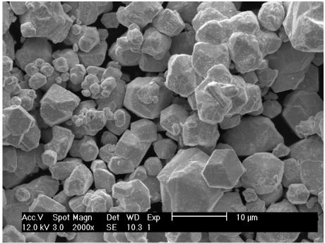
An SEM micrograph of tungsten powder. Note the angular nature of the particles and the agglomerations. The powder is produced by a multistep process where the final step is the reduction of tungsten oxide by hydrogen gas.
