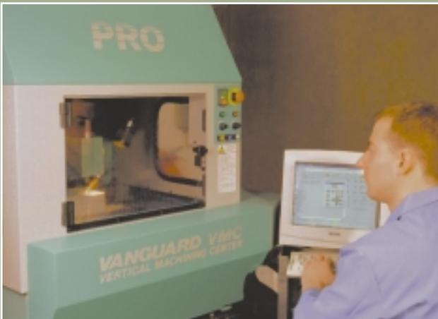
Pictured above - Jeremy Miller setting up the P/M lab's newest addition to rapid tooling - a high speed 3 axis CNC Milling Machine.
