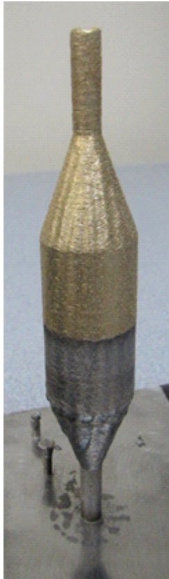
Figure 2: Near net shape cladding:- Tube is Inconel on the bottom and nickel-aluminum-bronze on the top. Courtesy: Applied Research Lab, Penn State
