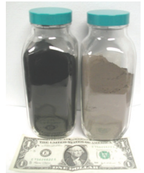
Figure 4.1: Unrefined and refined detonated nanodiamond powder with average particle size of 3-5nm
